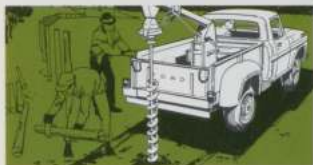
REAR-MOUNTED, PTO-DRIVEN MOBILE WORKSAVERS , such as post-hole diggers, feed mills, saw mills, hay balers, and other gear, belt or hydraulically actuated attachments are easily installed.
