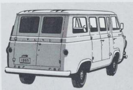
DISPLAY VAN. The Display Van has fixed windows in the right side for good lighting of bins, shelves, etc., which may be custom-built against the left wall. Vent-type right side door and fixed or vent-type rear door windows are available.
