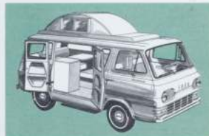
CAMPER. Convert to a Camper! Seats and sleeps six comfortably. To provide extra sleeping accommodations and increase headroom, you can add an elevating top which contains screened windows and a canvas bunk.
