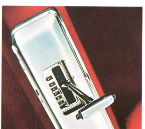
Sport Shift Merc-O-Matic is fully automatic when in "D" or a manual 1-2-3 shift. Available Cyclone GT only.
