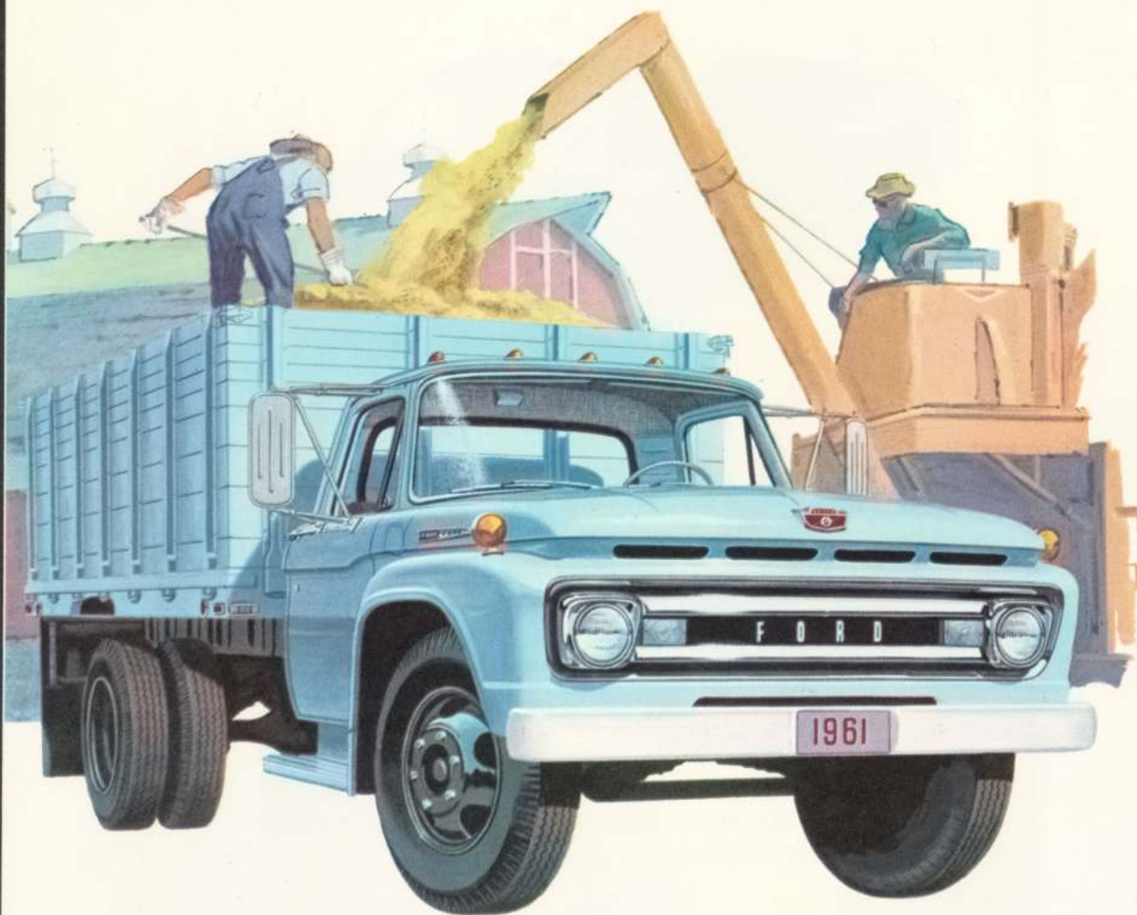
F-600 two-tonner offers a new power choice for '61, including the big all-truck 152-hp Six (available about Feb. 15). And the longer front and rear springs mean a smoother ride—without rubber-robbing independent front suspension.
