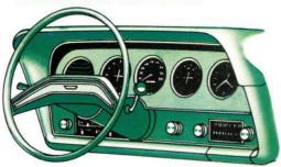
The LTD II instrument panel provides impressive driver convenience. All instrumentation and operating controls are driver-centered for easy viewing and reach. DirectAire Ventilation brings constantly changing fresh air to all occupants through instrument panel registers, even when all windows are closed.
