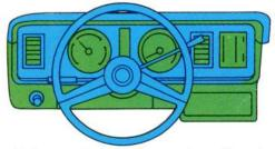
Driver-centered instruments and handy operating controls help keep the Fairmont driver on top of driving situations. Windshield wiper and washer functions are contained in one steering column lever, horn/turn signal/ headlight-dimmer functions in another.
