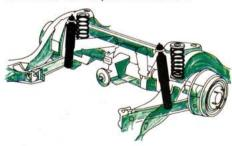
The rear suspension is a four bar link design incorporating coil springs centered over the axle with shock
