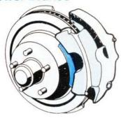
LTD II's heavy-duty power brakes are self-adjusting. Self-adjustment occurs automatically when the car is moving in reverse and the brakes are gently applied.
