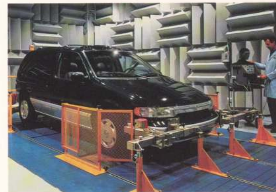
All-wheel-drive dynamometer chamber at the Advanced Engineering Center, Dearborn, Michigan
