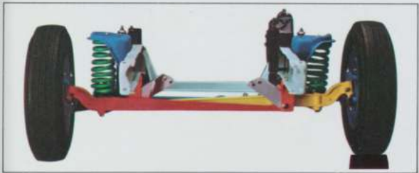
How Twin-I-Beam works. Front wheels operate independently, each on its own axle. Axles are forged steel I-beams, as used in big-truck axles. Forged steel radius rods secure axles to frame siderails maintaining wheel alignment. Axles and radius rods pivot in husky no-lube bushings.
