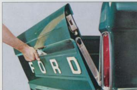
ONE-HAND TAILGATE LATCH. Pull—and the Ford Styleside tailgate opens. Push—and it snaps shut automatically. The single center tailgate latch releases the tailgate easily . . . only one hand does it.
