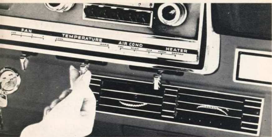
One finger tab controls warmth and coolness on built-in Fairlane air conditioner
