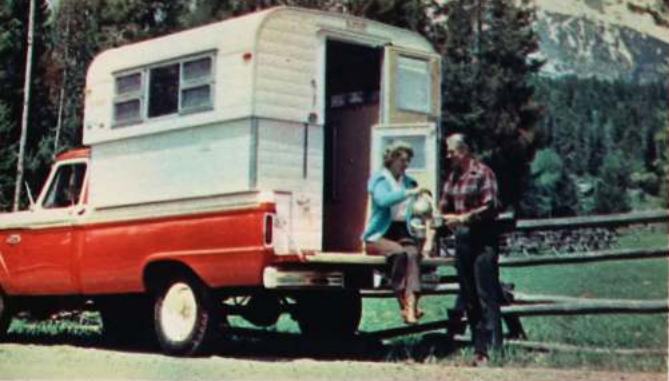
The Alaskan (left) elevates hydraulically for stand-up height. At right is kitchen area
