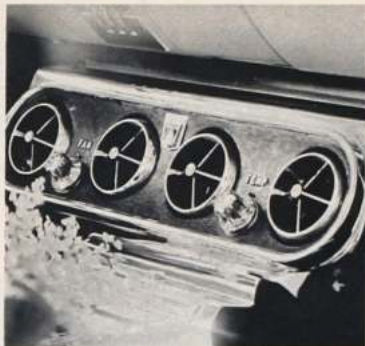
This is the Ford under-dash model, showing air ducts
