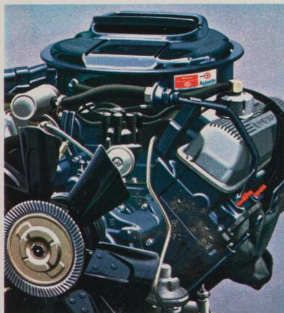
CJ 428 engine spews 335 horsepower with 440 lb. ft. of torque. 10.6:1 compression ratio. Huge 735 cfm capacity 4-barrel carburetor. Performance-tailored camshaft. Low-restriction air cleaner. Free-flow breathing characteristics.
