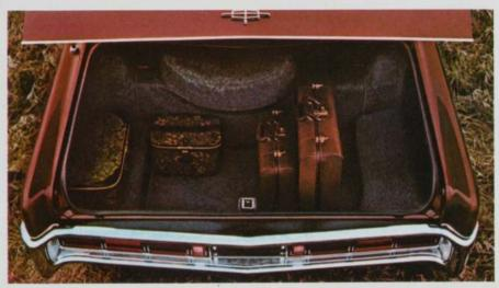
Continental's luggage compartment has a usable capacity of 18.1 cubic feet, fully carpeted. An optional remote-control deck-lid release includes a trunk-open warning light on the instrument panel. The tire cover is also optional.
