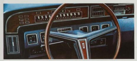
This new instrument cluster places the most-often-read dials—fuel and temperature—closest to the driver's line of vision. There are warning lights for headlamp doors closed, low fuel and dual brake system malfunction and a seat belt reminder light. The glove compartment has been doubled in size to accommodate many more of your travel accessories.
