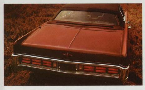
The all-new tail assembly reflects this motorcar's total sculptured elegance. The rear deck louvers are the outlet for Continental's new Flow-Thru Ventilation system. Very quietly and evenly, this system passes up to 480 cubic feet of fresh outside air through the passenger compartment every minute, even with all the side windows closed. You have full control of the air flow by means of switches within easy reach.
