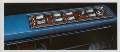
Padded armrest on driver's door organizes switches (left to right) for window and door locks; four power windows; power seat control and remote-control outside mirror.
