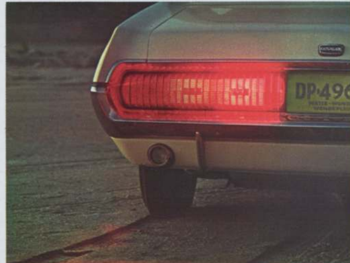
Sequential turn signals flash in a three-step movement.
