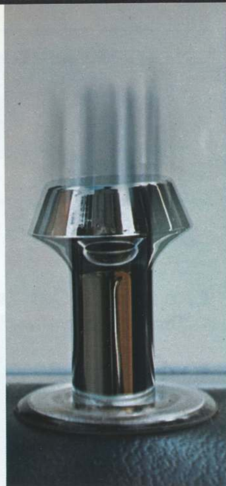
Speed-Actuated Power Door Locks—reach eight mph and all doors lock automatically.
