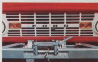
Front-Mounted Winch with 150 feet of 5/16-inch cable is power take-off driven.
