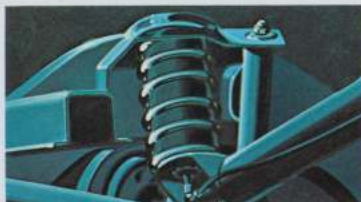
Automatic Load Leveler. Pressurized air bags in each rear spring automatically help keep car at a constant height from the road and level regardless of load.
