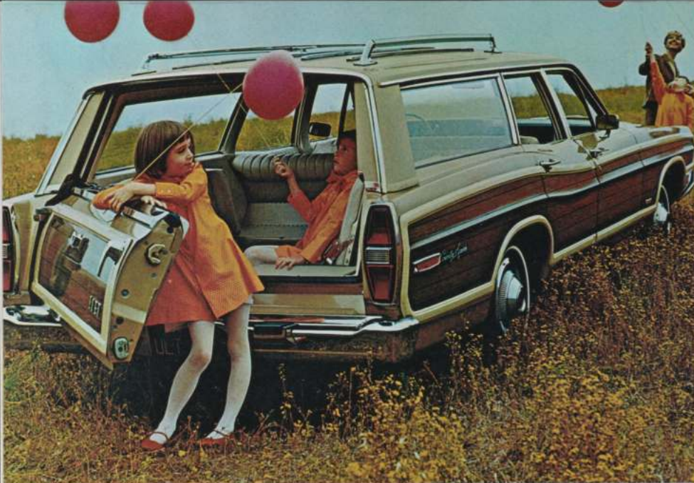
Magic Doorgate. Ingenious hinge design lets you swing Doorgate out like a door for passengers, or down like a tailgate for cargo. Standard on all Ford station wagons.
