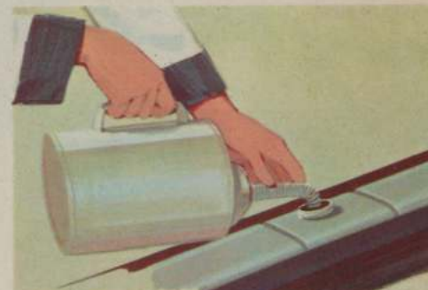
36,000-mile or 2-year, whichever comes first, long-life anti-rust, anti-freeze coolant—factory-installed coolant contains ethylene glycol concentrate and rust-inhibitor, gives you more carefree driving, regardless of weather.
