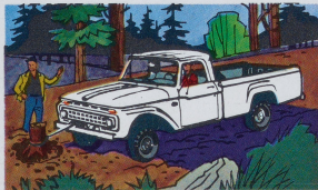
FRONT-MOUNTED PTO-DRIVEN winches, pumps, scoops, snow blades, etc., combined with 4 x 4 traction make light work of tough jobs. Engine power transmitted through a PTO drive does many jobs easily.
