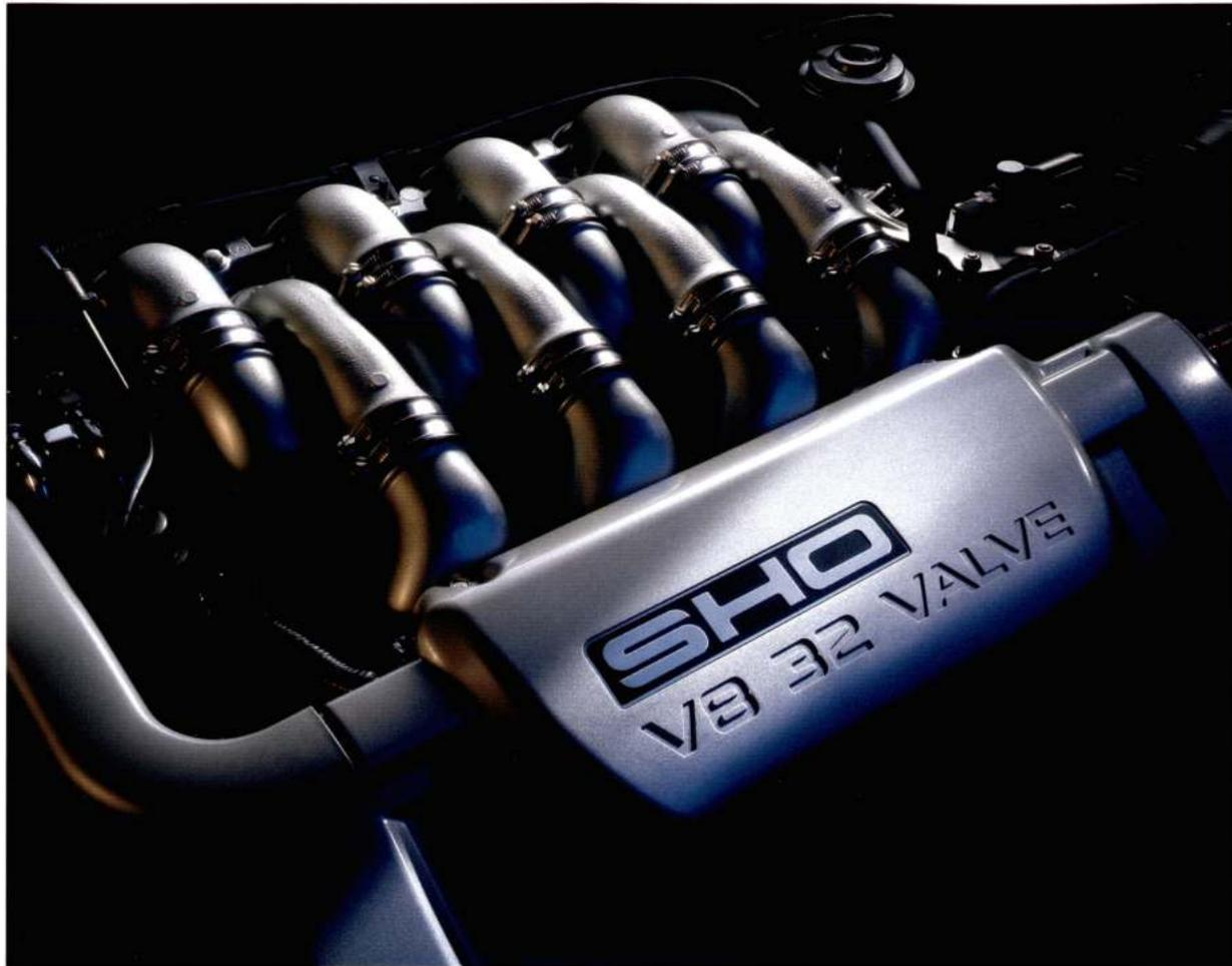
The heart of Taurus SHO is its sophisticated performance. A responsive electronic four-speed automatic overdrive transaxle, a special ride-adaptive suspension and a four-wheel disc anti-lock braking system are all standard. The new 3.4-liter 60-degree V8 engine has four valves per cylinder for free breathing. It produces 235 SAE net horsepower at 6,100 rpm and 230 foot-pounds of torque at 4,800 rpm.
