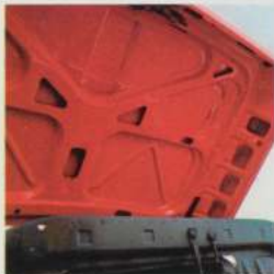
Double-wall section hood strength
