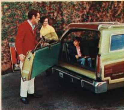
Ford-pioneered Magic Doorgate opens as a door with rear glass
