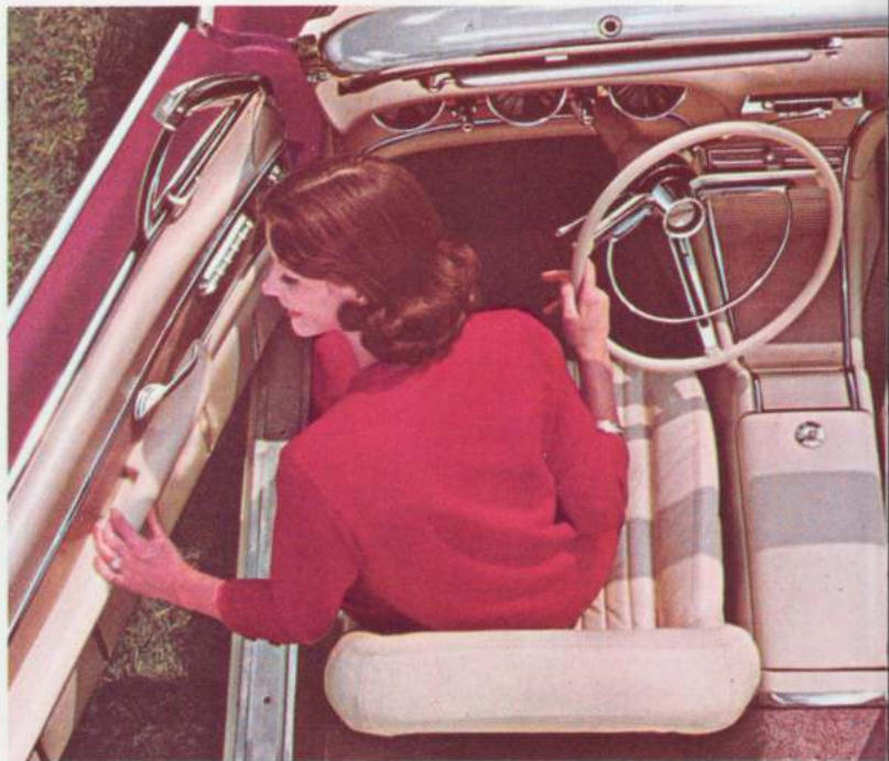
The wheel may be moved back to its normal driving position with the Cruise-O-Matic selector lever in "P" (Park). There are no other knobs or levers to operate.
