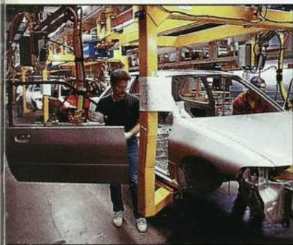
Workers at the Wayne, Michigan plant remove Escort doors to install instrument panels.
