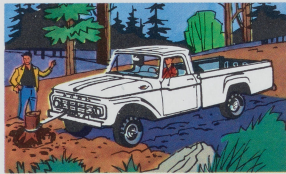
Front-mounted PTO-driven winches, pumps, scoops, snow blades, sweepers, etc., combined with 4 x 4 mobile power, make light work of tough jobs. Engine power is transmitted to do the job easier and faster.
